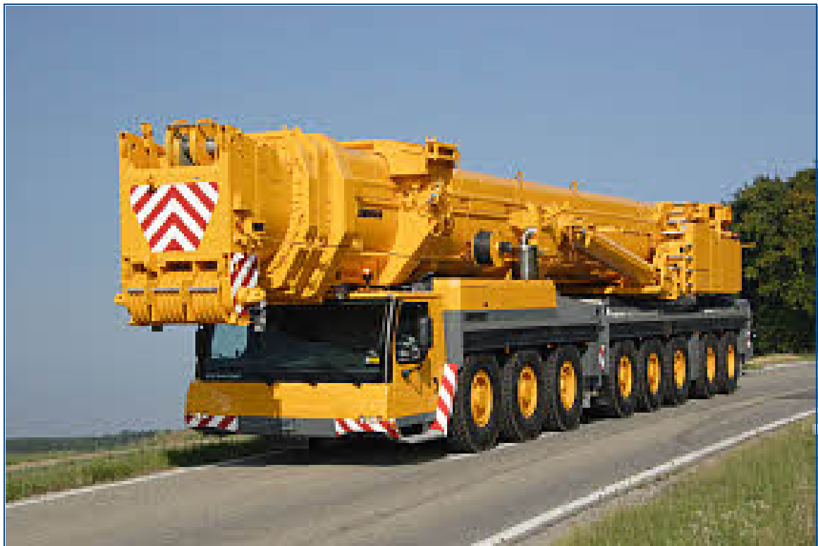
Figure 3.2: Crane for Wind Turbine Erection
